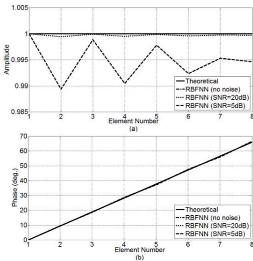
Fig. 2. The theoretical and RBFNN aperture distributions of a plane wave at  $\theta = 3^\circ$ : (a) the amplitude distribution and (b) the phase distribution.
