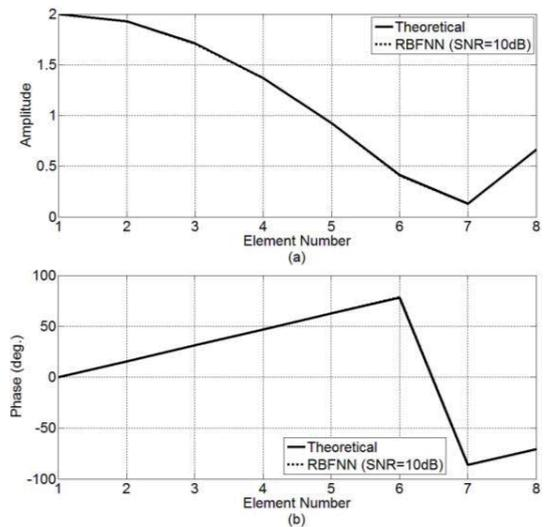
Fig. 3. The aperture distributions of a desired source at  $\theta = 0^\circ$  and an interferer at  $\theta = 10^\circ$ : (a) the amplitude distribution and (b) the phase distribution.
