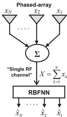
Fig. 1. Block diagram for phased-array data recovery using RBFNN.
